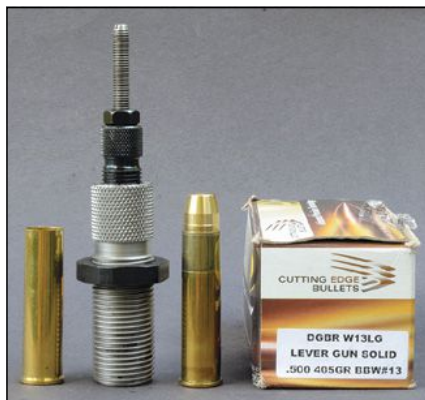
Running a Starline .50 Alaskan case (left) into an RCBS .50 B&M Alaskan full-length resizing die (center) necks it down for a .500-inch bullet (right).
