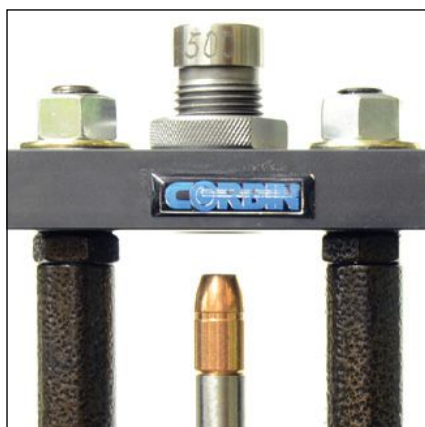
Using a Corbin CSP-1 press to push the Swift .510-inch, 450-grain A-Frame through an annular draw die decreases its diameter to .500 inch for the .50 B&M Alaskan.
