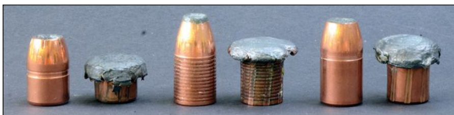
Pristine bullets and those recovered from expansion test media at 50-yard impact velocities include (left to right): a Swift 325-grain A-Frame, a North Fork 450 Bonded SP and a Swift 450 A-Frame.
